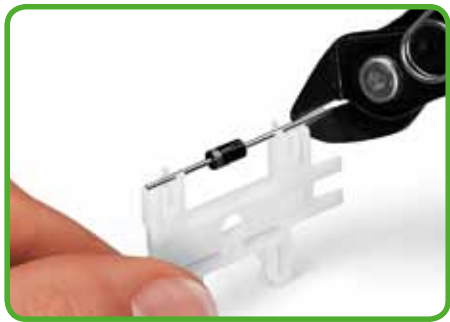
Measure component length with 2002-116 tool
